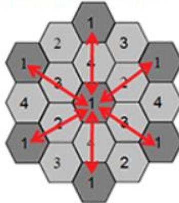
Increased Frequency Reuse (w/ 80 MHz channels) - All same-channel BSS blocking
