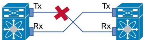
Figure 48. UniDirectional Link Detection (UDLD)
