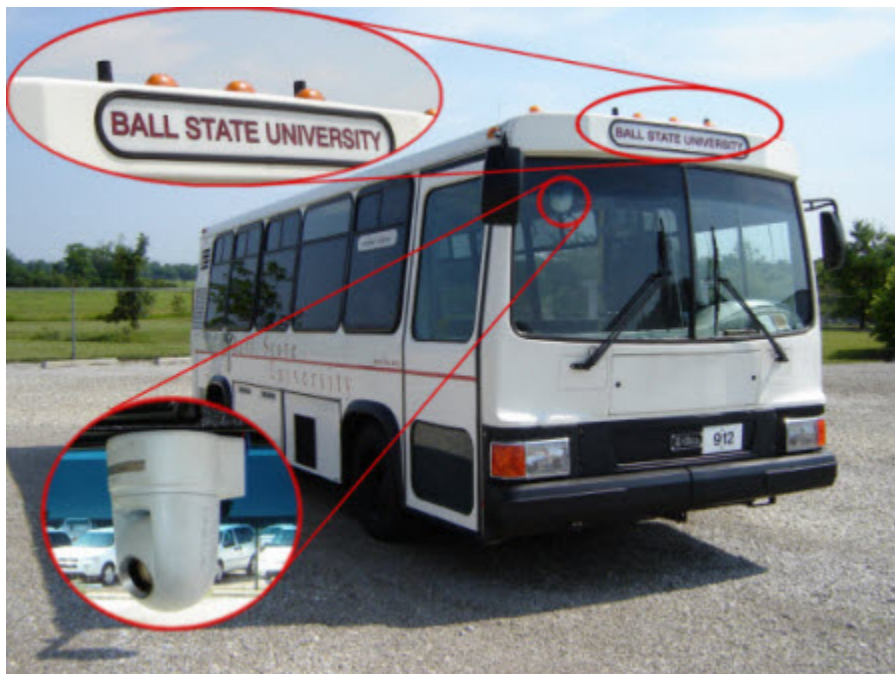
Ball State University Shuttle Bus with WiMAX enabled GPS & Video Camera
