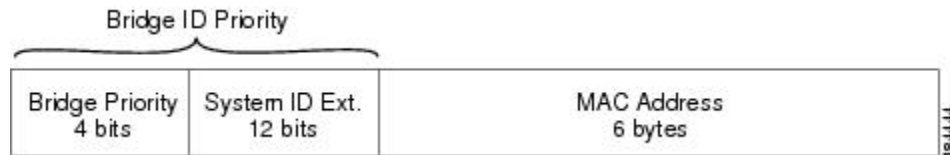
Figure 12: Bridge ID with Extended System ID
