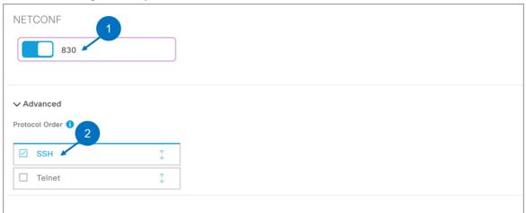
4. Check Cisco DNA Center discovery result to see Cat9300 discovered: The "NETCONF" discovery is essential to be successful for enabling embedded 9800 on the Catalyst 9300 switch.
