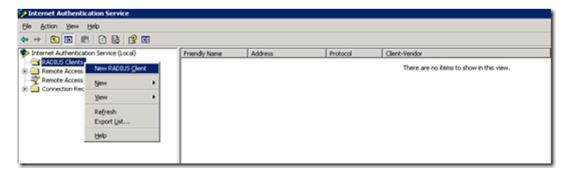
On the New Radius Client window enter a name for the RADIUS client as well as the devices IP Address. Then press NEXT.
