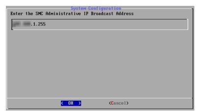
The IP Broadcast Address page opens with the default broadcast IP address.
