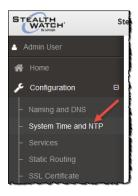
The NTP Server page opens showing the NTP server that you set in the initial configuration using the Appliance Setup Tool.
