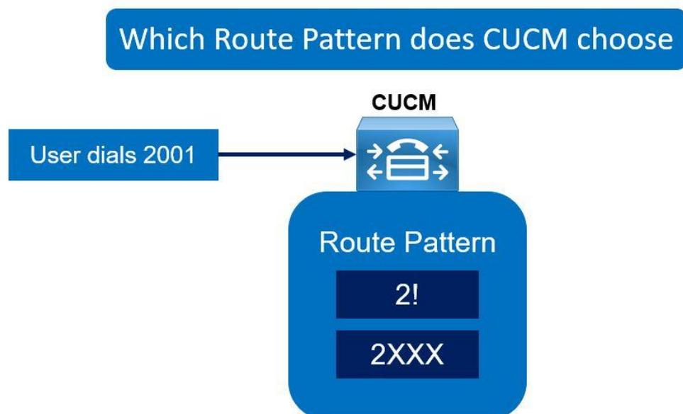
Route Pattern the **2!** pattern matches an infinite number of digits because the pattern matches a variable number of digits but for the purposes of closest-match routing, digit
