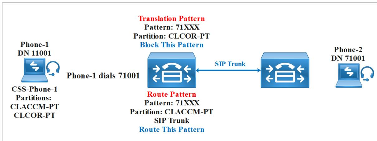
The **Phone-2** will ring because when we have equals match in this case a Translation Pattern and a Route Pattern then CUCM uses higher Partition in CSS (the Partition listed first). In this case **CLACCM-PT** is higher than **CLCOR-PT** so it will match the Route Pattern and will routes the call. So the **Phone-2** will ring because the RP is listed first in the partitions list.
