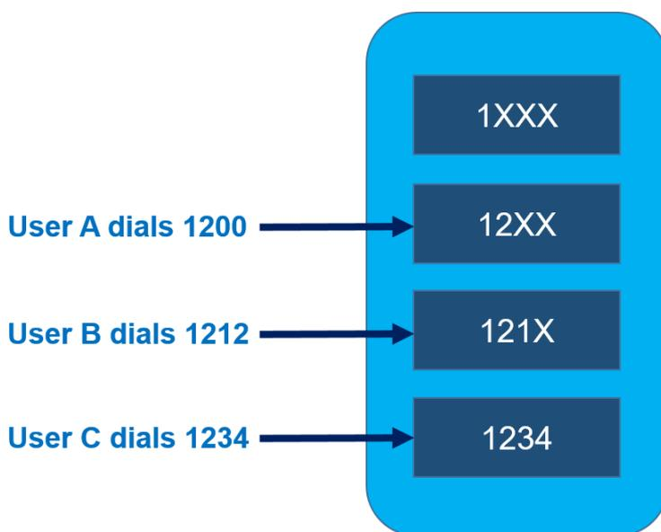
When User A dials the string **1200**, Cisco Unified Communications Manager compares it to the patterns in its call-routing table. In this case, there are two potentially matching patterns: **1XXX** and **12XX**. Both of these patterns match the dialed string, but **1XXX** matches a total of 1000 strings (from **1000** to **1999**), whereas **12XX** matches only 100 strings (from **1200** to **1299**).
