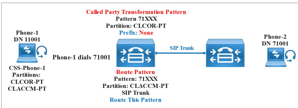
The **Phone-2** will not ring. The Called Transformation Pattern is applied after the route-pattern decision and after the Gateway or SIP Trunk Selection. Here what happen, the **Phone-1** CSS has access to the Called Transformation Pattern Partition, this Partition is listed first, the result is that there is a blackhole. and the call will not be routed.
