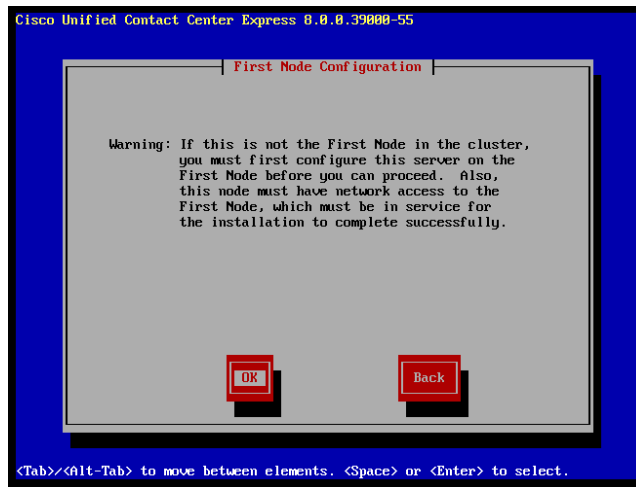
Figure 16 First Node Configuration Window with Warning Message
