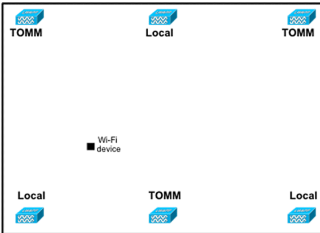
Figure 10: Tracking Optimized Monitor Mode AP deployment
