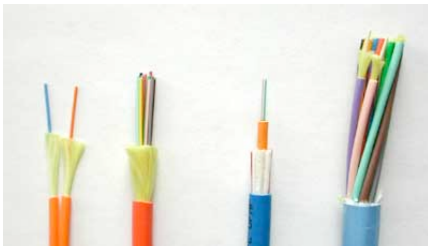
Cables (L>R): Zipcord, Distribution, Loose Tube, Breakout
