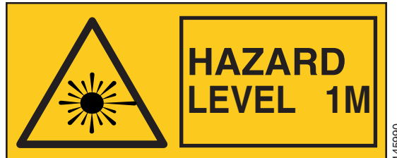
Figure 11-2 Hazard Level Label
