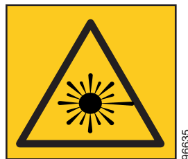
Figure 11-3 Laser Source Connector Label
