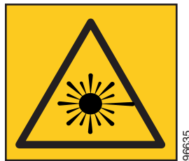
Figure 12-8 Laser Source Connector Label
