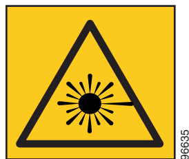
Figure 7-8 Laser Source Connector Label
