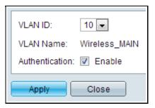
Step 15. check Enable to allow authentication on that VLAN and click Apply. Repeat for each VLAN.
