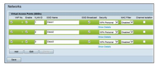
**Note**: The default SSID for VAP0 is ciscosb. Every additional VAP created has a blank SSID name. The SSIDs for all VAPs can be configured to other values.
