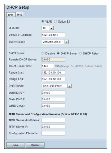
Step 4. In the VLAN ID drop box, select the VLAN you are setting up the address pool for (in this example VLANs 10, 20, and 30).
