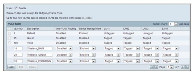
Step 2. We are creating 3 separate VLANs to represent different target audiences. Click **Add** to add a new line and edit the VLAN ID and Description. You will also need to make sure that the VLAN is set to Tagged on any interfaces that they will need to travel on.
