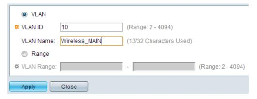
Step 3. Enter the VLAN ID and the VLAN Name (use the same as the description from Section I). Click Apply, and then repeat this step for VLANs 20 and 30.
