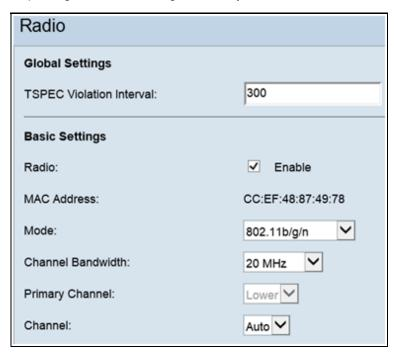
Step 2. Click the **Enable** check box to enable the Wireless Radio.
