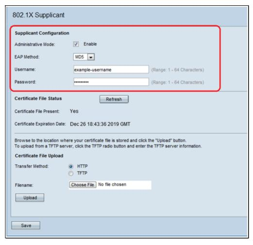
Step 9. Check **Enable** in the Administrative Mode field to enable the device to act as a supplicant in 802.1X authentication.
