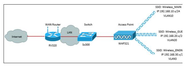
The image above illustrates a sample implementation for Wireless access using multiple SSIDs with a Cisco small business WAP, switch and router. The WAP connects to the switch and uses the trunk interface to transport multiple VLAN packets. The switch connects to the WAN router through the trunk interface and the WAN router performs inter-VLAN routing. The WAN router connects to the Internet. All wireless devices connect to the WAP.
