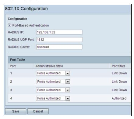
Step 8. Enable Port-Based Authentication and configure the IP address of the server.
