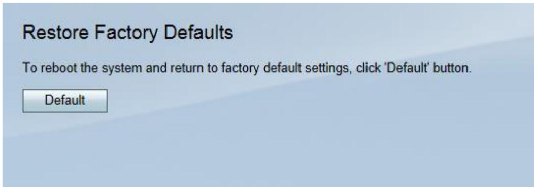
Step 2. To reset the device, click the **Default** button. This will erase all current configurations.
