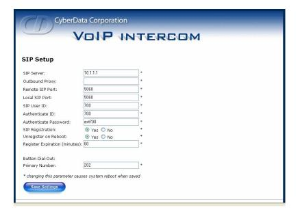
These parameters have a corresponding setting on the UC500/CME Device:
