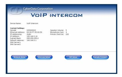
The above page shows the current configuration on the Callbox. Please write down the MAC address, as it will be needed later for configuring the UC500/CME device.
