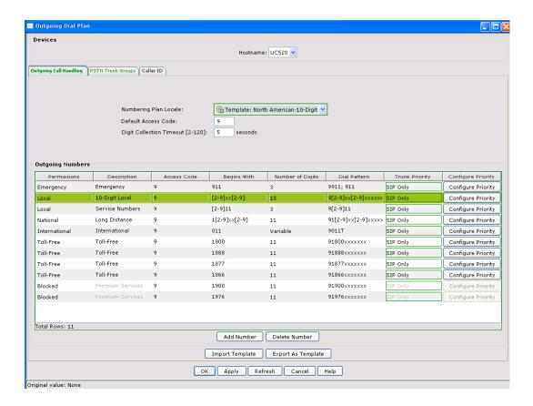
4) Click on **Add Number** to insert the entry for calls to the QuesCom gateway. Ensure that the **Permissions** selection is also correct for the users that will be placing calls through the gateway:
