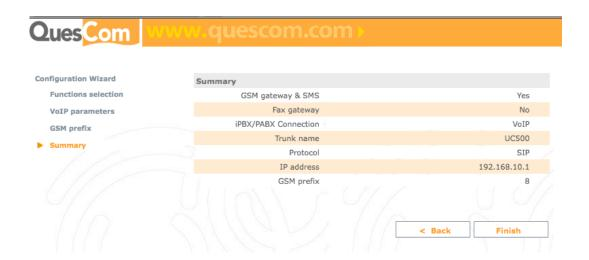
At this point, the gateway is ready to receive calls from the UC 500 and send them to the mobile network accordingly. It is still necessary to configure the UC 500 side, which we will be doing next.
