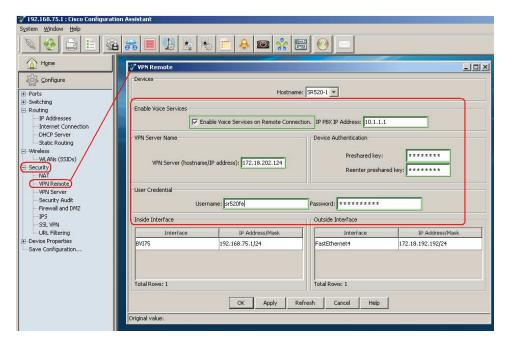
After applying, release / renew you PC IP address and then SAVE the CCA SR520 config using CCA SAVE ICON!!!
