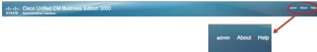
**Step 2** The About link provides a fast way to determine the software version and licensed organization associated with the BE 3000 unit. Version 8.6.1 is shown in this example. Click the “X” in the upper corner of the About window to dismiss it.
