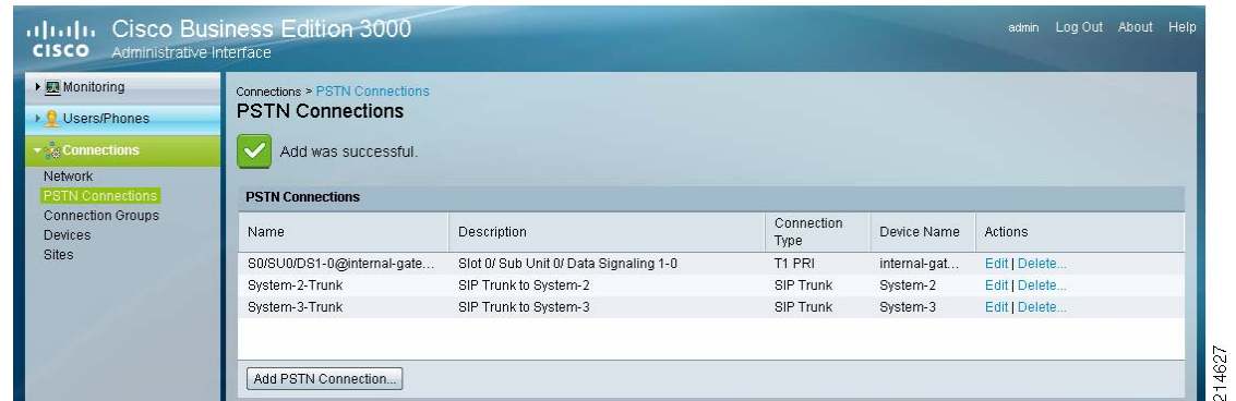
Figure 9 Listing of SIP Trunks and External PSTN Connection
