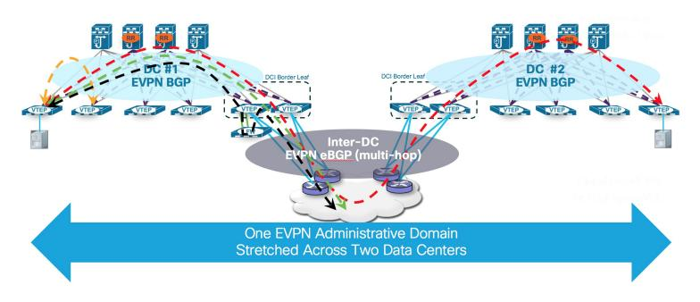
In this use case, each tenant will extend their layer 2 network across a layer 3 underlay network using VXLAN. For example, a host that is part of Room A will be able to create a virtual layer 2
