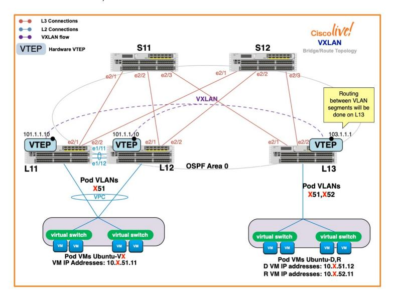
The hardware based external VXLAN solution lab (a host in the datacenter communicating with a host outside of the datacenter [on the internet, for example]) is setup based on the following network topology (this is an excerpt of the master physical topology shown earlier – only datacenter A and the external/firewall portion is included):
