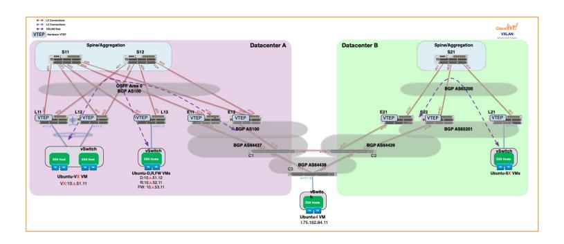
As was discussed earlier, DC A is using OSPF for the underlay and IBGP for the overlay. DC B, however, will be using EBGP for both the underlay and overlay to demonstrate another way to configure VXLAN.
