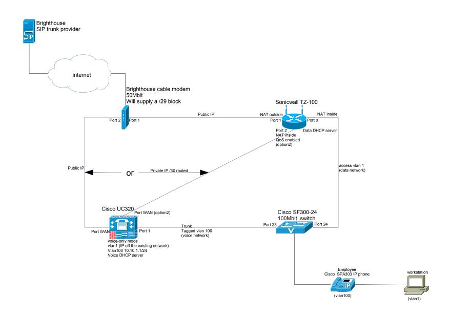
**Voice only** (using pre-existing VLAN and DHCP server for data)—The UC300 device is added as a voice appliance in a fully functional pre-existing network. In the greyfield voice-only scenario, the voice VLAN is not seen by the router of the pre-existing network. The voice VLAN terminates on the UC300 device, while the data VLAN terminates on the existing router.
