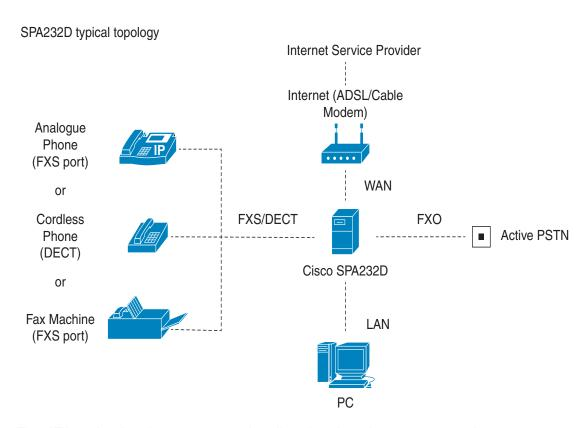
The ATA maintains the state of each call and makes the proper reaction to user input events (such as on/off hook or hook flash). Because the ATA uses the Session Initiation Protocol (SIP), it is compatible with most Internet Telephony Service Provider (ITSP) offerings.
