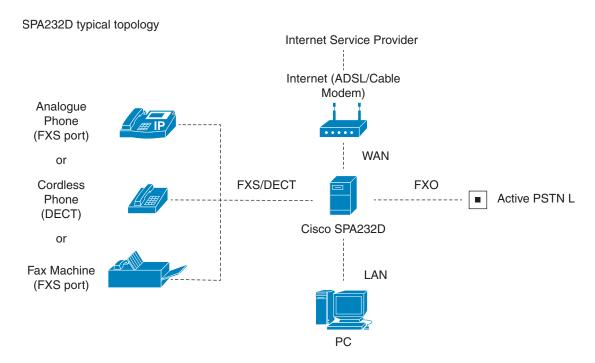
The ATA maintains the state of each call and makes the proper reaction to user input events (such as on/off hook or hook flash). Because the ATA uses the Session Initiation Protocol (SIP), it is compatible with most Internet Telephony Service Provider (ITSP) offerings.
