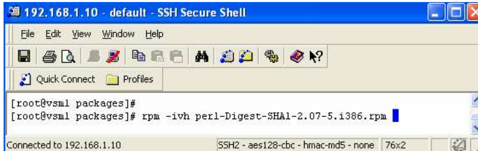
Figure 50 - Installing perl-Digest-SHA1 RPM
