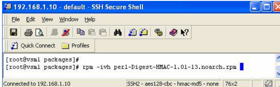
Figure 51 - Installing perl-Digest-HMAC RPM
