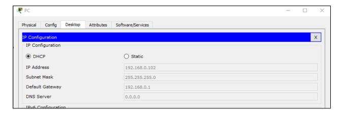
Click on the Command Prompt icon. Verify the PC has received an IPv4 address by issuing the ipconfig /all command from the Command as shown in the figure. The PC should receive an IPv4 address in the 192.168.0.x range.
