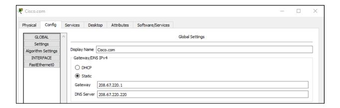
d. Configure the Cisco.com server FastEthernet0 Interface settings.
