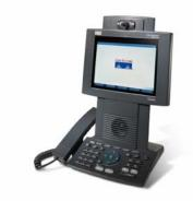
many accessibility methods based on user preference. In addition to the four functional buttons that provide access to Directories, Services, Settings, and Messages, the Cisco IP Phone 7985G has five buttons that control video features: Self View, Picture in Picture, Video Mute, Display, and Brightness.
