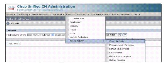
**Note:** In order to get the phone load name from CallManager 4.x, go to **System** > **Device Defaults** > **Device Defaults Configuration** and copy the load information.
