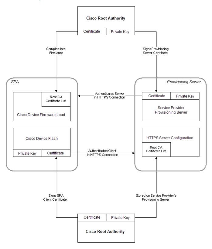
As indicated in the lower half of the diagram, a Cisco Small Business Client Certificate Root Authority signs each unique certificate. The corresponding root certificate is made available to service providers for client authentication purposes.
