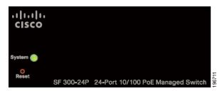
The switch can be reset by inserting a pin or paper clip into the reset opening. See "Returning the Device to the Factory Default Settings" for details.
