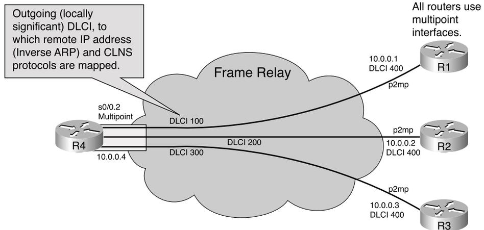
In Figure S-23, the network is still a star topology, as in the previous example. In a multipoint environment it is important that a full mesh be implemented; therefore, all routers in this network must have VCs interconnecting them, although these are not shown in the figure.
