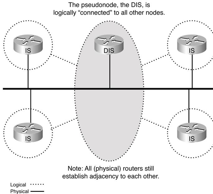
In IS-IS, all routers on the LAN establish adjacencies with all other routers and with the DIS. Thus, if the DIS fails, another router can take over immediately with little or no impact on the topology of the network.
