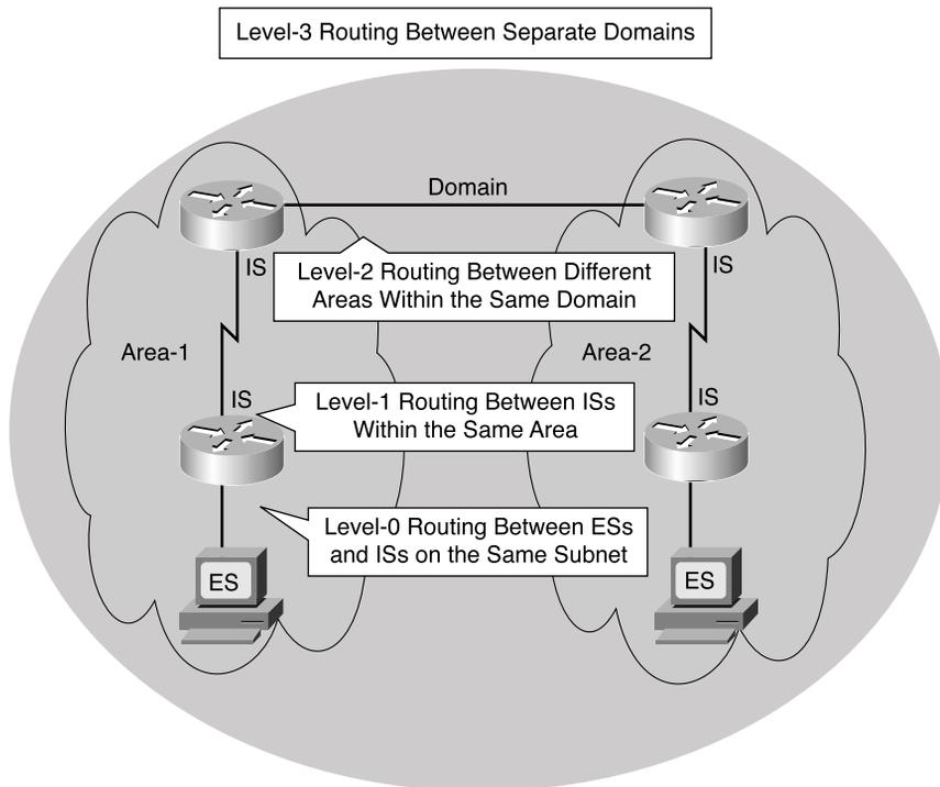
To simplify router design and operation, OSI distinguishes among Level 1, Level 2, and Level 3 routing. Level 1 ISs communicate with other Level 1 ISs in the same area. Level 2 ISs route between Level 1 areas and form an intradomain routing backbone. Level 3 routing is done between separate domains. Hierarchical routing simplifies backbone design because Level 1 ISs need to know only how to get to the nearest Level 2 IS.
