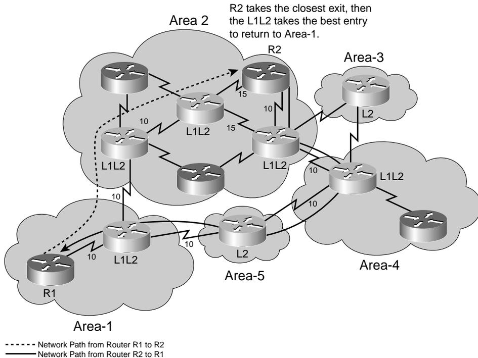
In Figure S-17, router R1 routes packets to router R2 through area 1's Level 1–2 router. This router looks at the destination area of the packet and routes it directly into area 2. In area 2, the packets are routed as Level 1 to R2 (even though the initial next hop is another Level 1–2 router, the routing is Level 1.)
