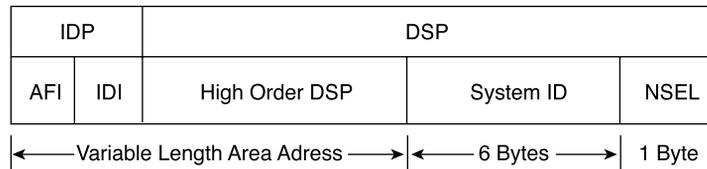
An OSI NSAP address can be up to 20 octets long and consists of the following parts, as shown in Figure S-6:
