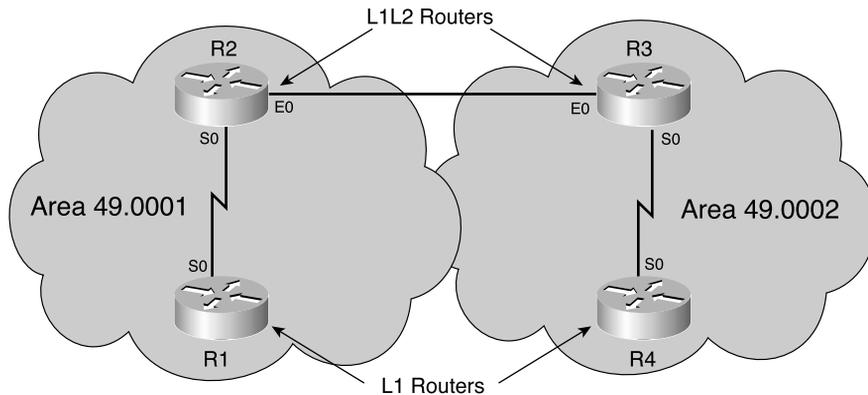
In Figure S-20, router R1 is in area 49.0001 with no links outside that area and, therefore, needs to operate only as a Level 1 router. The configuration for R1 is shown in Example S-11.
