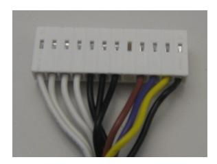
5) Reinstall this cable between the router's system board and the power supply along with the un-modified 4-pin blue ILP cable.
