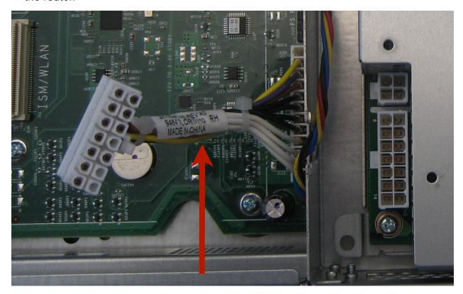
2) Locate the pin that needs to be removed. It is the black wire that is to the left of the brown wire:
