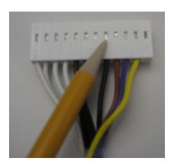
3) Insert a small slotted screwdriver in the slot for this pin and gently pull the wire out of the harness:
