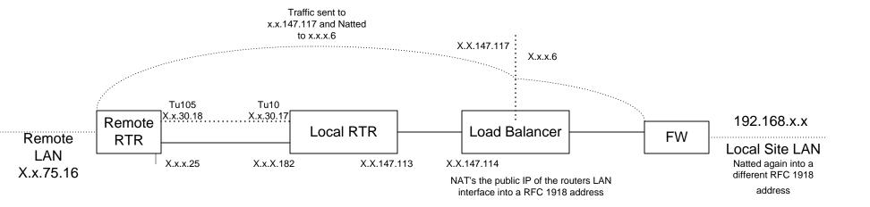
The Remote site router can ping x.x.147.117 (which is natted to x.x.x.6 going to the LAN)
