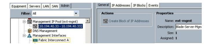
In the following screen it is shown that chassis-1/blade-1 is assigned the 10.194.40.33 IP address for remote KVM and virtual media access.
