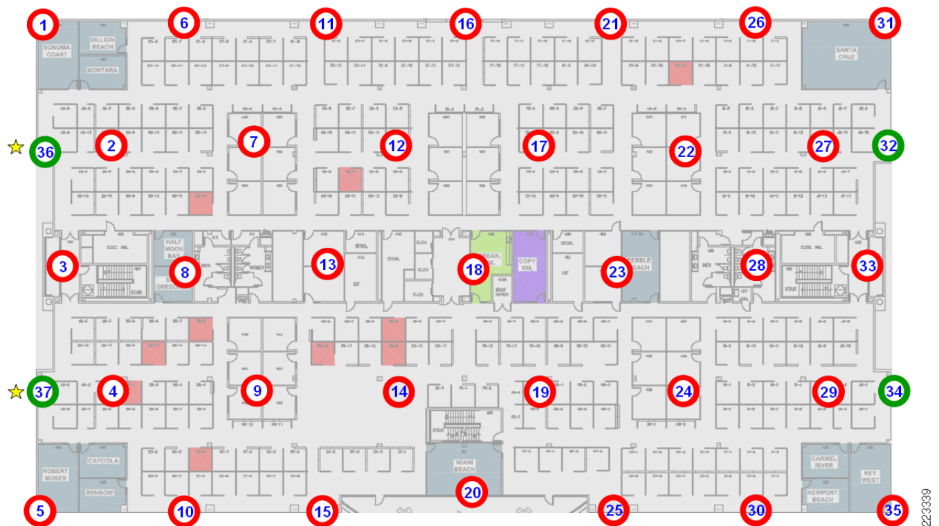
Figure D-3 Layout for 5GHz Voice and High Speed Data—2.4GHz Legacy with Location
