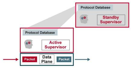
In summary of the stateful protocol feature, the high-availability switchover performance is more dependent on the status of the synchronization procedure than on the complexity of the configuration. After the system and protocols reach a stable operating point, the protocol state databases on each of the supervisors will have a fairly similar status. The resulting high-availability supervisor engine switchover performance is less than 3 seconds.
