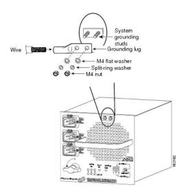
Additional information about system grounding can be found in the *Catalyst 6500 Series Switch Installation Guide* on cisco.com .
