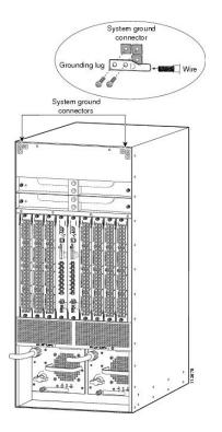
Due to the size of the 8700W power supply, it may cover up the grounding points on the 6506 and 6509 chassis. As a result, a grounding point was added to the 8700W power supply as seen in the following picture.
