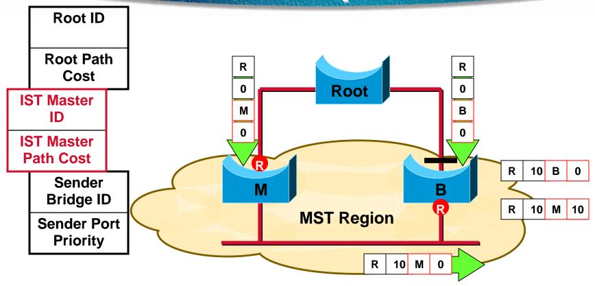
Result: the BPDU received by B inside the region is now better than the one received directly from the Root
