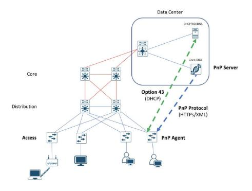
Cisco DNA Center is designed for intent-based networking (IBN). The solution breaks the process in to Day 0 and Day N. The solution provides a unified approach to provision enterprise networks comprised of Cisco routers, switches, and wireless devices with a near zero touch deployment experience.
