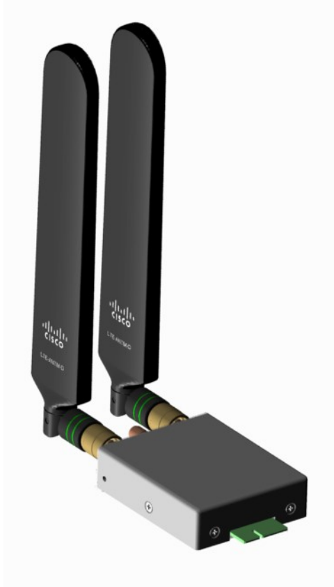
Figure 9: LTE Pluggable Module (with antennas)
