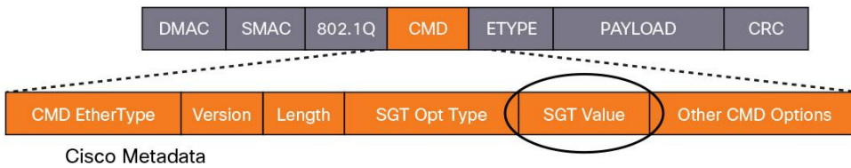
Figure 15. Layer-2 Frame Format with SGT
