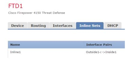
Since we have a trunk port going through FTD where the vlans do not change, we apply differentiated policy using the VLAN id. Traffic that belongs to inside1 uses VLAN id 920 and traffic that belongs to Inside2 uses VLAN id 925 so any rule created specifically for one or the other simply needs to include the VLAN id in the rule for it to be specific to one or the other.
