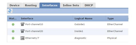
In the Inline Set area, we pair up the two port channels, Outside1 and Inside1 to form Inline1.
