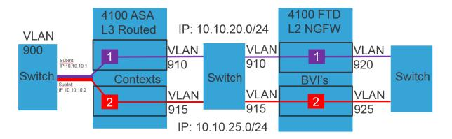
Hosts and services on either VLAN 920 or 925 can talk to the outside world on VLAN 900 and beyond and have a L3/L4 policy built in an ASA context and zone-based FTD policy for application, content and threat related protections. This scalable NGFW solution enforces traffic isolation between contexts/BVIs, and allows FTD policy separation by using security zones and FMC ACP categories.
