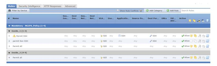
Zones can be used to provide an additional layer of functionality by allowing inbound or outbound policies. By creating a North Zone with the port channels from ASA to FTD and a South Zone with port channels from FTD to Switch, one can enforce directionality on policy allowing the admin to create policies specific to traffic coming from outside to inside vs traffic going from inside to outside.
