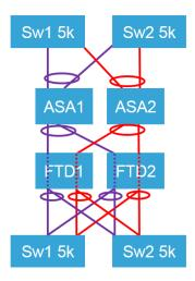
The end result is that ASA passes traffic off on a trunk port carrying VLAN's 920 and 925 and because these trunk ports are going through interface paired ports on FTD, they are not modified and exit FTD on
