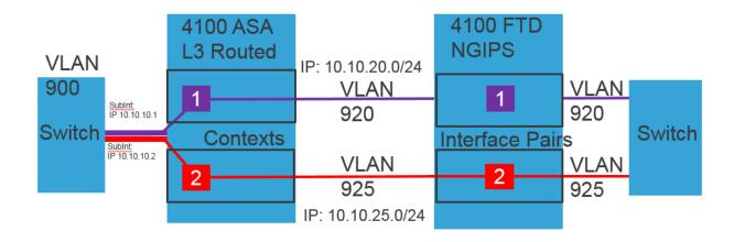
Hosts and services on either VLAN 920 or 925 can talk to the outside world on VLAN 900 and beyond and have a L3/L4 policy built in an ASA context and VLAN based FTD policy for application, content and threat related protections. This Resilient+ NGFW solution enforces traffic isolation between contexts/VLANs, and allows FTD policy separation by using VLANs and FMC ACP categories.
