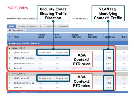
Reviewing the Resilient+ NGFW Design with Active Standby ASA contexts and FTD clustered interface pairs enforcing independent traffic paths and differentiated policy. The logical packet flow is documented below:
