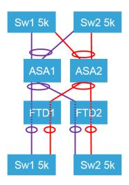
Because ASA is in active standby HA, either all packets will traverse the purple path, or in the case of a failover, all packets would then be moved to the red path. In any case, because both ASA and FTD are deployed with state sharing all flows are handled statefully. The port channel to the cluster allows the active ASA to send all of the traffic headed inbound to be load balanced across all the FTD instances in the cluster.
