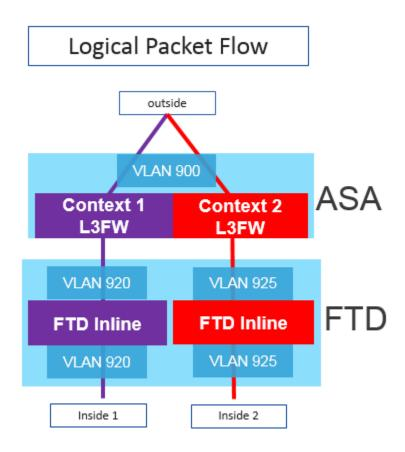
Since we have a trunk port going through FTD where the VLANs do not change, we apply differentiated policy using the VLAN id. Traffic that belongs to inside1 uses VLAN id 920 and traffic that belongs to Inside2 uses VLAN id 925 so any rule created specifically for one or the other simply needs to include the VLAN id in the rule for it to be specific to one or the other.
