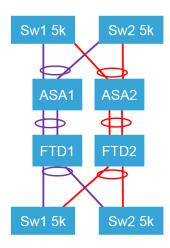
The result is that ASA passes traffic off on trunk port carrying VLAN's 920 and 925 and because these trunk ports are going through interface paired ports on FTD, they are not modified and exit FTD on the same VLANs they entered on. Interface pairing ensures traffic segregation because the flow of packets is unaltered and remain on the VLANs they entered on without any ability to have them put on different VLANs.
