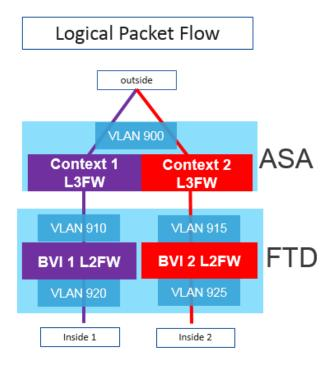
Additional controls in terms of policies can be imposed by using security zones and their assignment into dedicated ACP rules for each BVI. If we define a security zone per BVI sub-interface, we can then build policy rules that are specific to the BVIs. The following FMC screenshot shows assignment of security zones to their appropriate BVI port-channel sub-interface.
