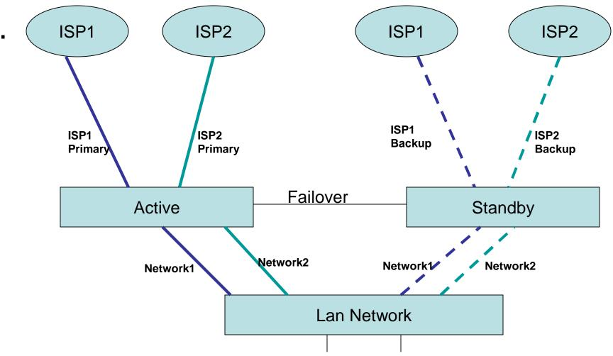
Network 1 uses ISP1 Primary link during normal operation and ISP1 Backup link during failover Network 2 uses ISP2 Primary link during normal operation and ISP2 Backup link during failover
