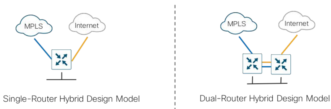
Figure 14 Single-router and dual-router hybrid design models
