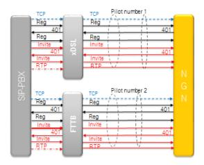
Figure 8-1: Redundant trunk registration (N=2) – simplified flow
