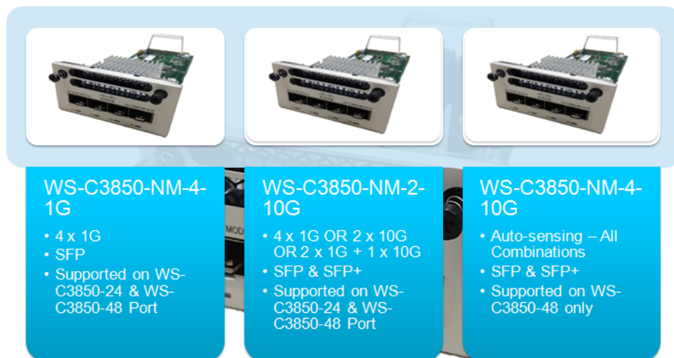
Figure 79. Catalyst 3850 Network Modules
