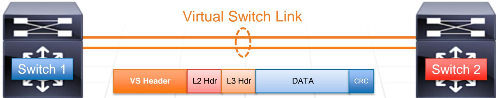
All traffic traversing the VSL is encapsulated into a 32 Byte **Virtual Switch Header (VSH)**
