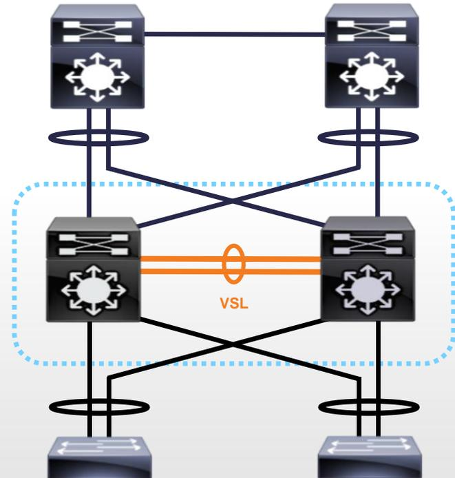
Recommend to deploy the VSL with **2 or more** links, distributed across multiple Line Cards to ensure the highest redundancy
