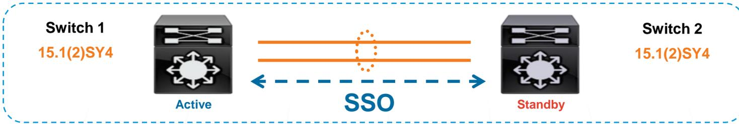
If a **mismatch** occurs between the Active & Standby, the Standby will revert to **RPR mode**
