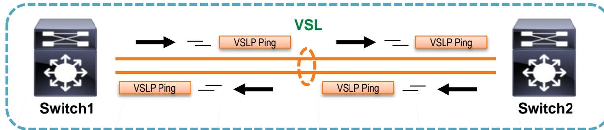
VSLP Ping operates on a **per-physical interface** basis and parameters such as COUNT, DESTINATION, SIZE, TIMEOUT may also be specified...
