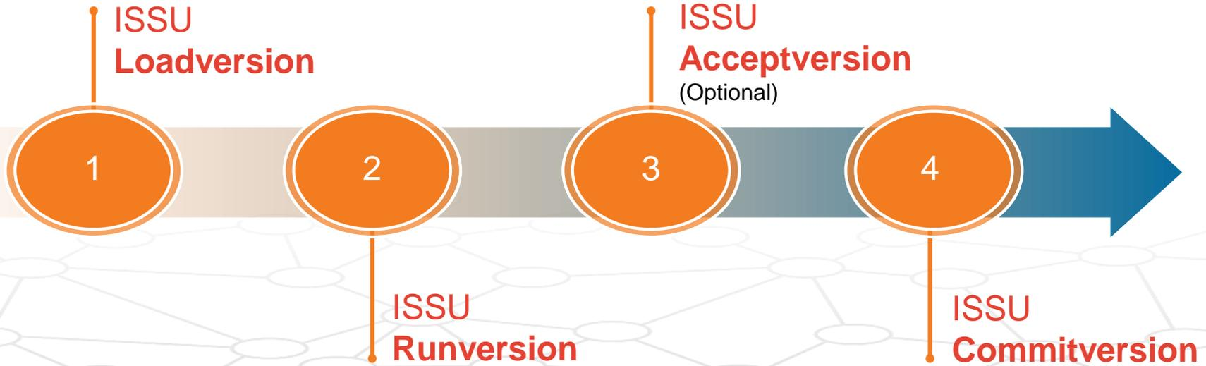
The ISSU Process in VSS is referred to as **Enhanced Fast Software Upgrade (EFSU)**
