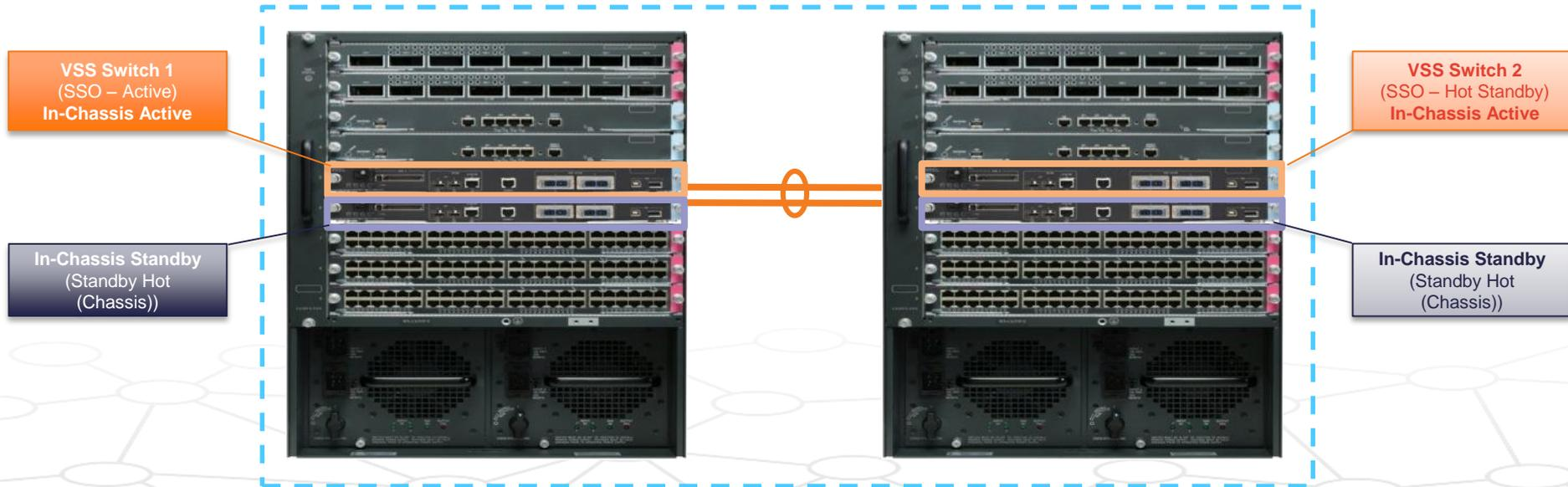
**STANDBY HOT (CHASSIS)** is a new redundancy mode created for the VSS ICS Supervisor
