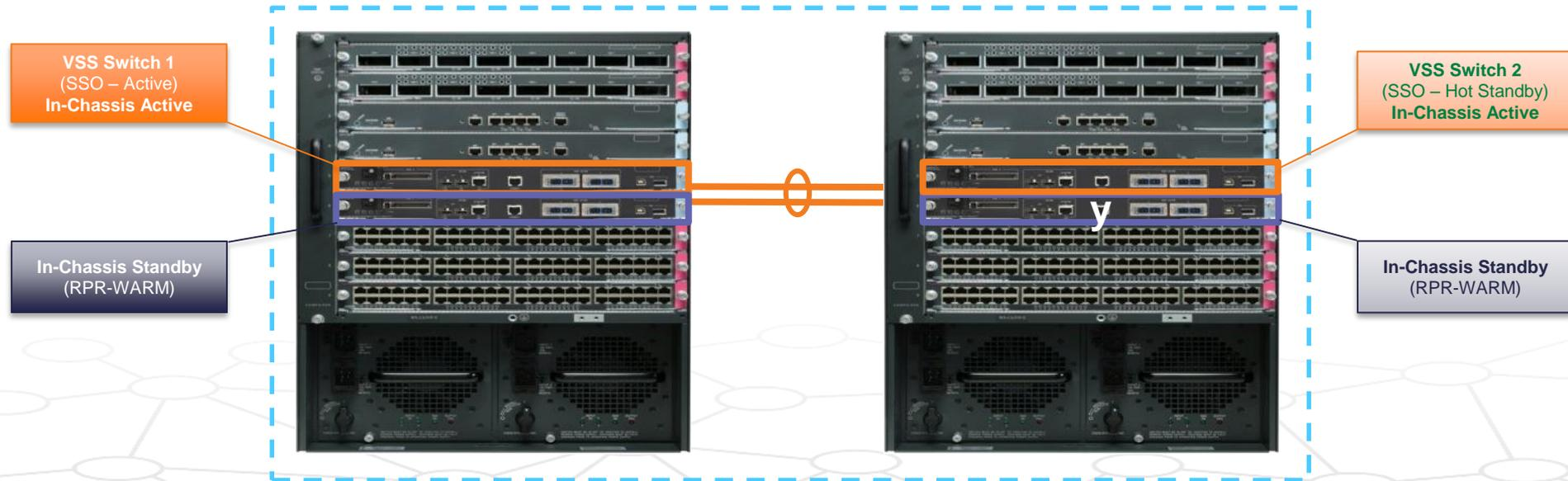
**RPR-WARM** is a new redundancy mode created for the VSS In-Chassis Standby Supervisor
