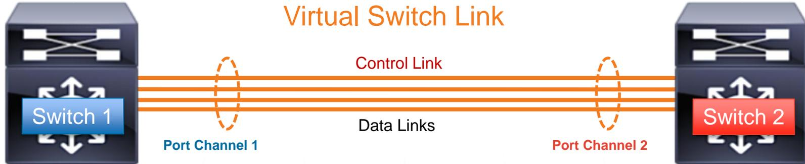
Just as other Port Channels, one link is selected as a “Control Link”, for the purpose of transmitting BPDUs and Port Channel status.
