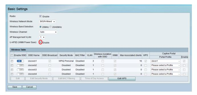
Step 8. In the *Wireless Table* area, check the check boxes corresponding to the SSIDs you want to configure. You can edit multiple SSIDs at the same time.
