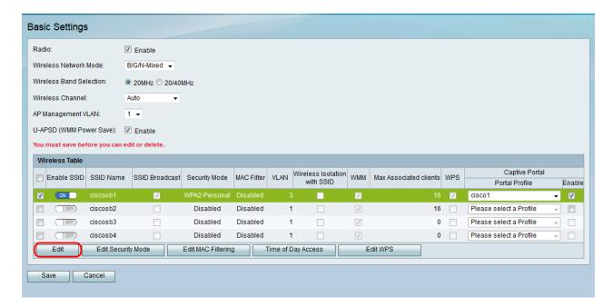
Step 10. Enable the desired SSID by changing the I/O slider to **ON**.
