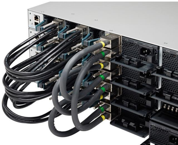
Figure 5. StackWise-480 and StackPower Connectors
