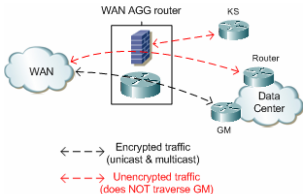
Figure 4-5: Encrypted Traffic to the GM Bypasses a Firewall
