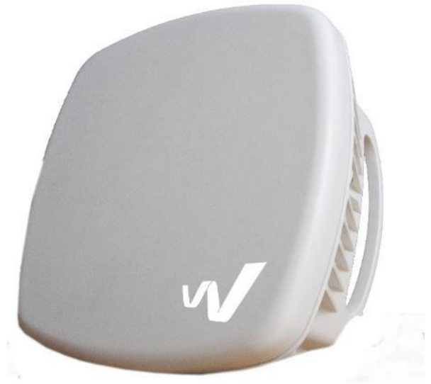
Figure 2. Bluwan's LinkFusion Metro NTE is a 15 x 15 cm high-capacity terminal for small cells. Source: Bluwan
