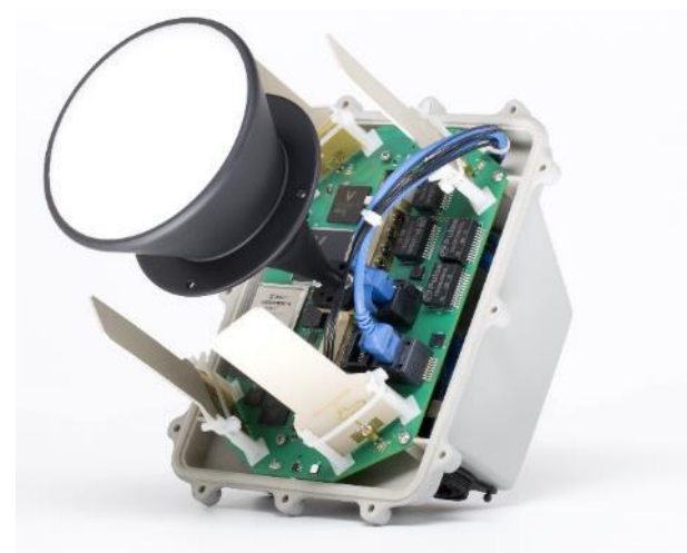
Figure 2. HaulPass micro SC 5/60 GHz small cell wireless backhaul system. Antennas are fixed. Source: VubIQ
