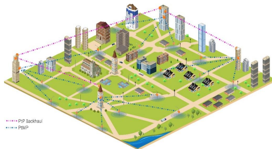
Figure 18. Tsunami 8200 NLOS backhaul systems used in PTP and PMP small-cell backhaul applications, providing up to 250 mbps throughput. Source: Proxim
