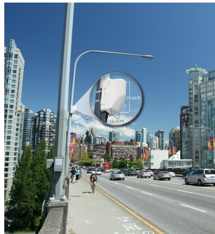
Figure 17. StreetNode area-licensed PMP microwave backhaul system for small cells featuring automatic antenna alignment.
