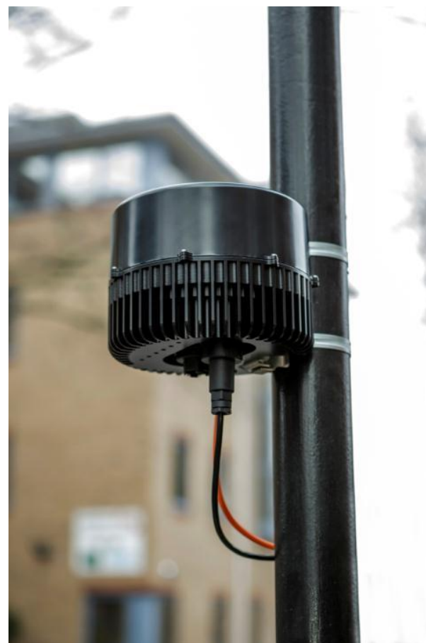
Figure 13. CCS MPTMP area-licensed microwave backhaul terminal for small cells. Source: CCS
