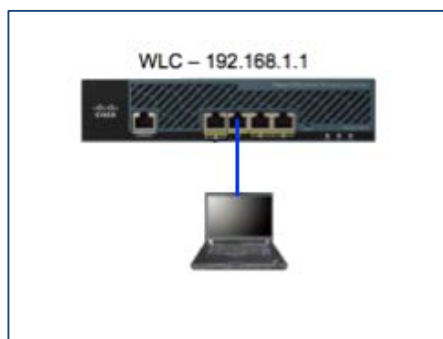
Figure 5 Connect Laptop to WLC
