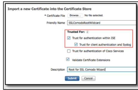
Figure 71 Import a new Certificate into the store
