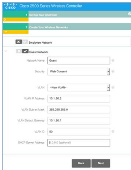
Figure 7 Create Your Wireless Network
